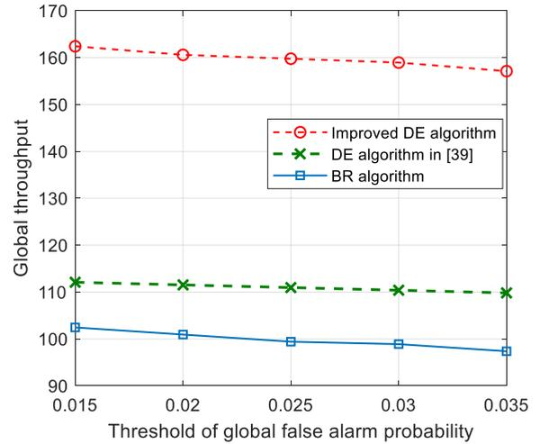
**FIGURE 11. Global throughput vs. the threshold of global false alarm probability in different algorithms.**
