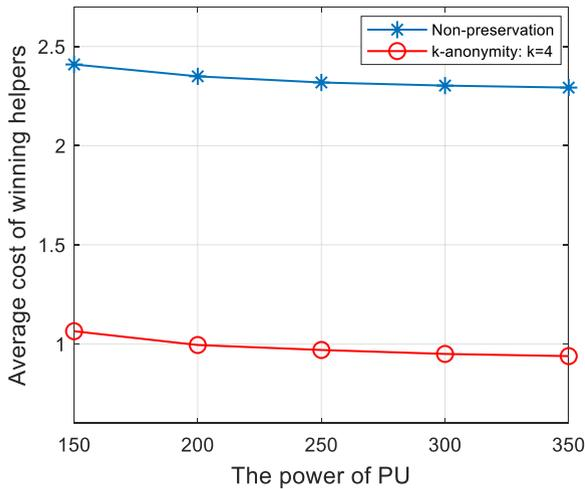
FIGURE 5. Average cost of winning helpers vs. the power of PU in  $k$ -anonymity and non-preservation mechanism.
