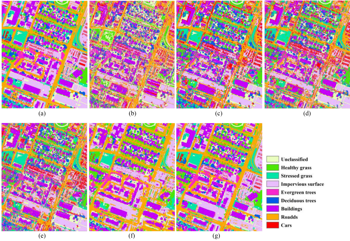
Fig. 10. Classification results of grss_dfc_2018 data with different neural network algorithms. (a) Ground truth map. (b) 2-D CNN. (c) 3-D CNN. (d) PCA-CNN. (e) 3-D-ResNet. (f) DeepLabv3. (g) Proposed method.
