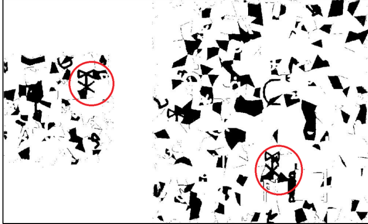
Figure 46: An example of a monochromatic image produced by color histogram. In this image there is a matching pair which is connected to its surrounding similar-color background noise and was not detected by the recognition algorithm.
