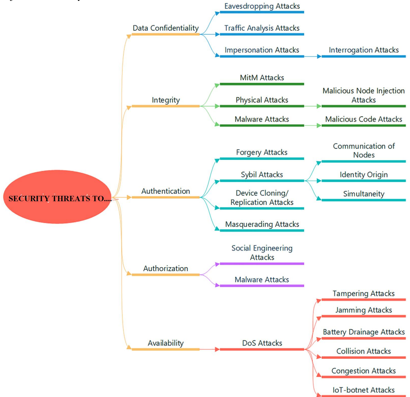
Figure 69: - Security threats in IoMT network [74]
