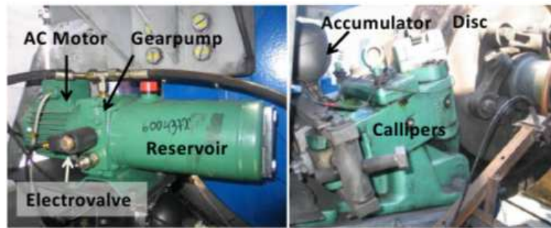
Figure 8. Example of wind turbine brake system [24] [24]
