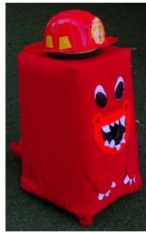
Fig. 1. DragonFlu: a remotely driven, mobile, table tennis ball launcher. Balls are thrown from the mouth upon command from a remote app. The robot can move, driven by moving the phone/tablet where the app runs.
