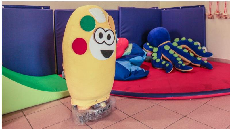
Fig. 3. The mobile robot Teo, presented in the playing environment. The coloured patches can be substituted by others functional to question-answers games. The eye expression and mouth can also be selected by the player to customize the emotional aspect of the robot.
