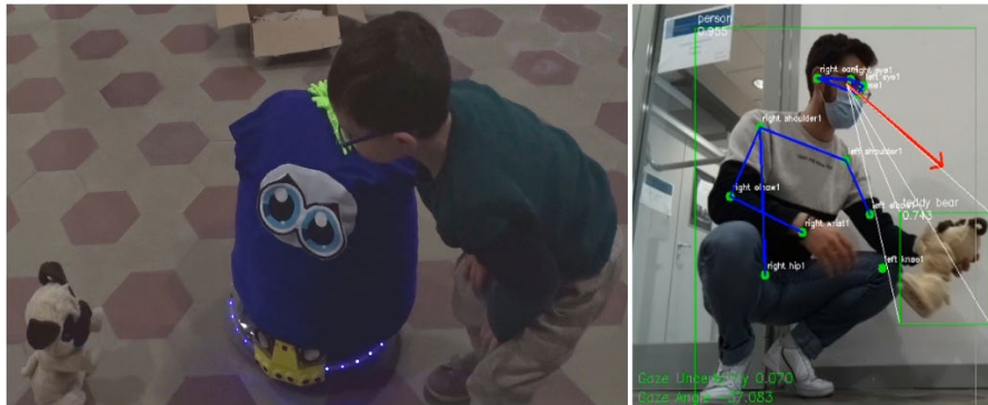
Fig. 2. (a) The mobile robot OIMI in action attracting the attention of the player to the puppet on the left. (b) The skeleton and sight direction detection from OIMI’s camera images.
