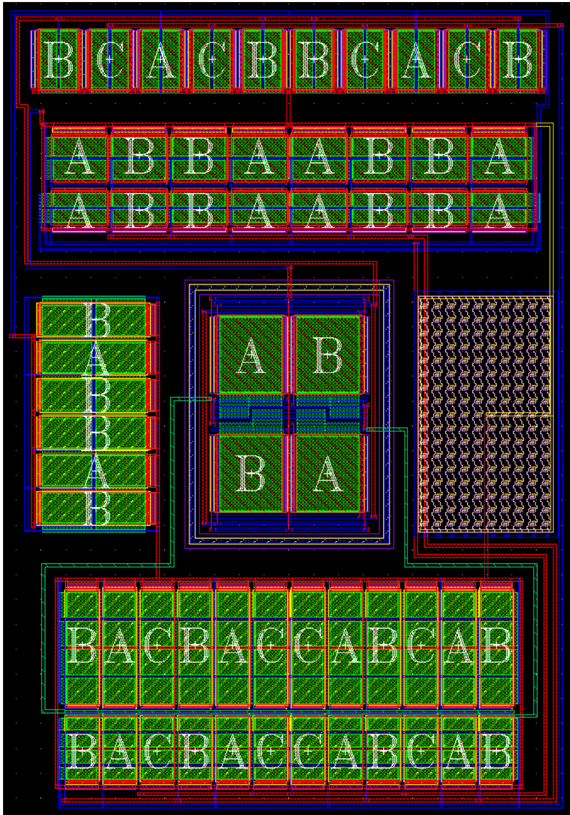
Figure 8.20: Finalized layout of the Folded Cascode OTA, obtained by SWARM for a 2:3 aspect ratio.
