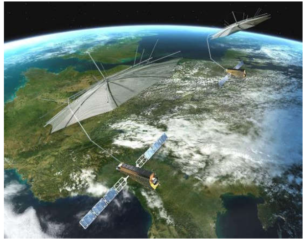
Fig. 3. Artist's impression of the Tandem-L satellite twins flying in close formation. The single-pass interferometric mode with adjustable across-track baselines is especially tomographic imaging of volume scatterers.
