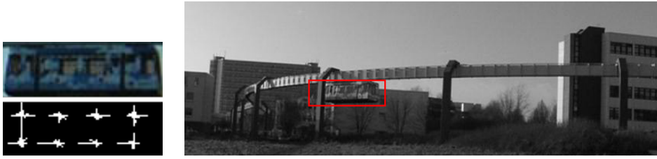
Figure 2.9: Example of a HoG detector. (left) a foreground sample and its HoG descriptor. (right) An exemplary detection of the object.
