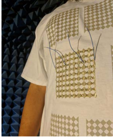
Figure 5.6.7: Photo of RF harvesting T-shirt with an 81-element rectenna array. Courtesy of José Estrada.
