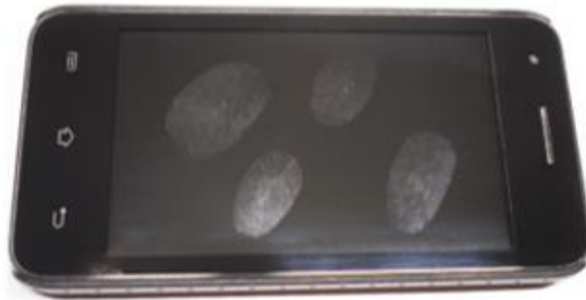
Figure 23. Latent fingerprints left on the surface by tapping the genuine user's finger.
