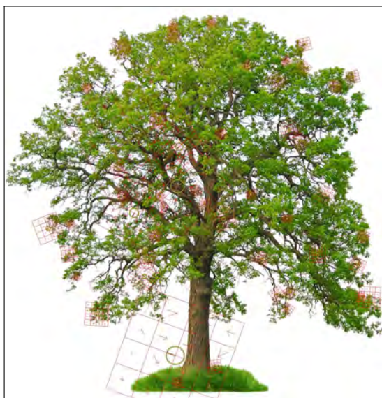
Figure A.8: Sample SIFT feature detection in a drawing of a tree. The different sizes of the descriptors correspond to features detected at different scales.
