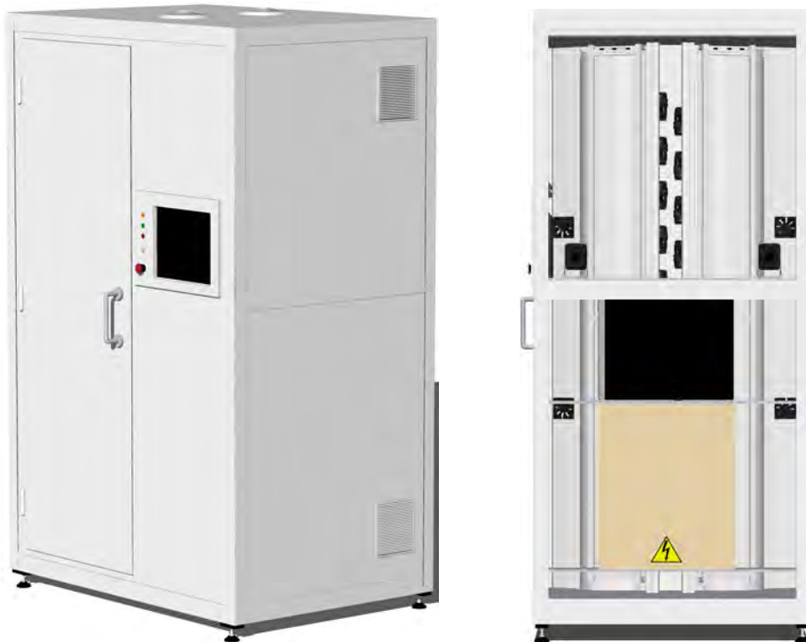
Figure 3.2: Exterior view of the scanner (3D model): the equipment compartment. At the bottom and the top of the side paneling there are ventilation openings for air intake and exhaust. The interior of the equipment compartment can be seen in the image on the right (the two parts of the composite paneling are removed). There are three shelves holding the equipment cabinet, the PC, and the stereo speakers. Behind the shelves are the camera rig, the lighting system and the intake fans facing the interior of the acquisition chamber.
