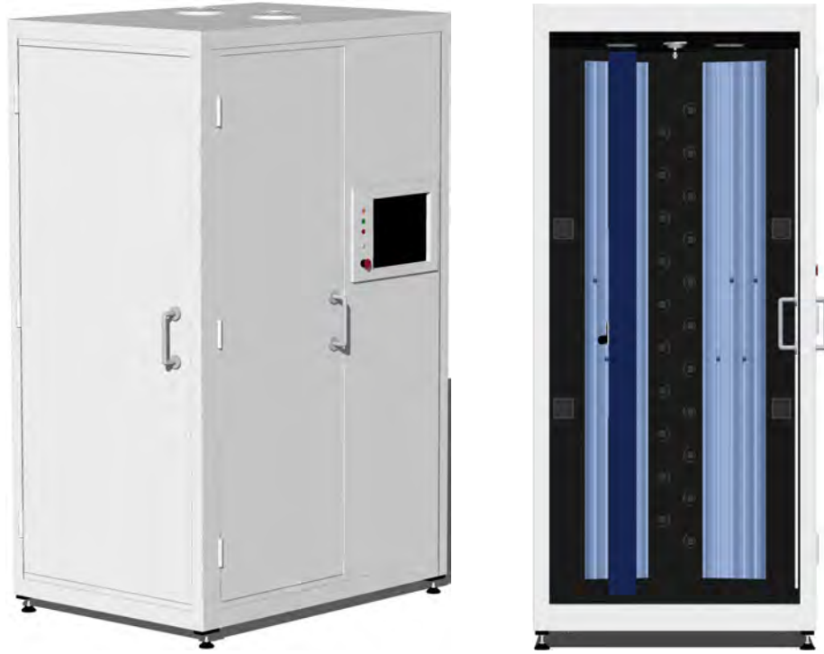
Figure 3.1: Exterior view of the scanner (3D model): the acquisition compartment. The two doors allow for easy entrance and exit regardless of the position of the backrest column. The control panel is located next to the front door and consists of a touchscreen, emergency stop button and operation LEDs. The interior of the acquisition chamber is shown in the image on the right (the side door removed). The camera rig is covered by black paneling and located in the middle of the cabin. On the side of the rig, there are the two sections of the lighting system as well as the four intake fans. The backrest column, padded with soft blue material, is attached to the turntable at the bottom and to the roof frame at the top.
