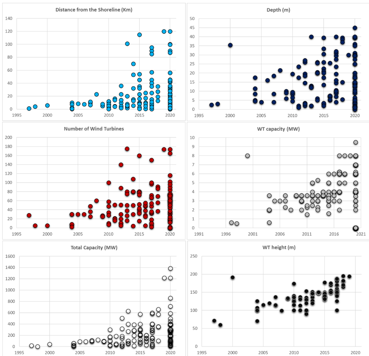
Figure 2.1.2: Distance from the shore, Depth, Number of WTs, WT capacity, Total OWF capacity and WT hub height (from the sea bottom) evolution from 1995 - 2020
