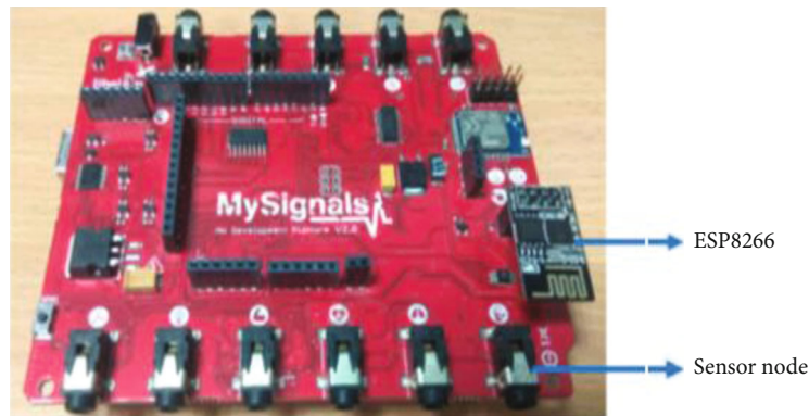
FIGURE 8: MySignals with sensor nodes and WiFi module.
