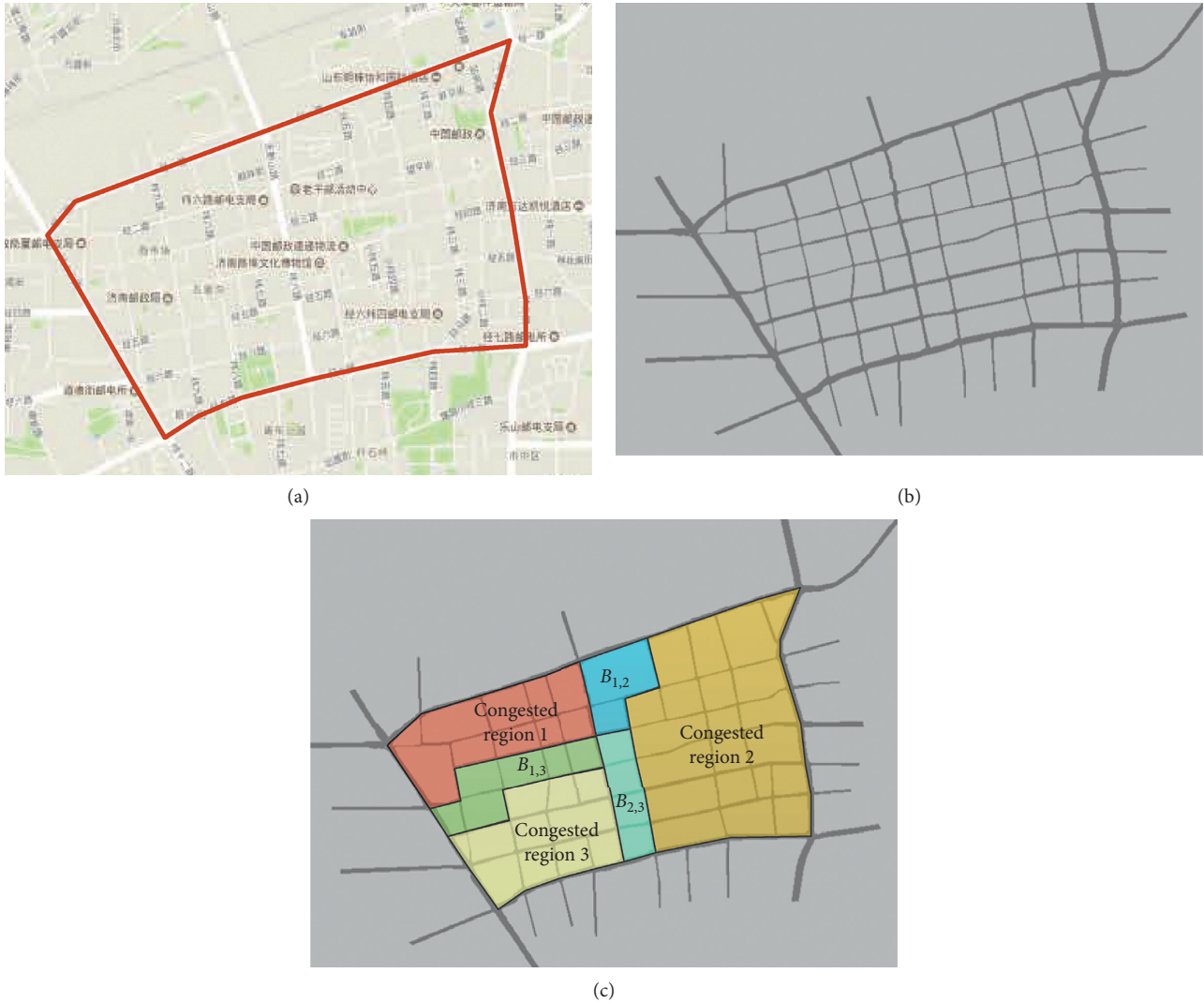
FIGURE 4: The test site of downtown Jinan: (a) real network, (b) simulation model, and (c) partitioning of the network into 3 congested regions and 3 boundary regions.
