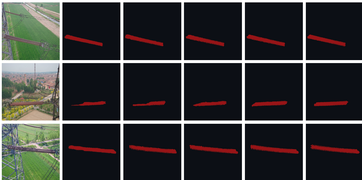
FIGURE 8: Examples of semantic segmentation results on insulator test dataset. (a) Original input image; (b) the predicted image of Base Module; (c) the predicted image of the former combined with CAM; (d) the predicted image of the former combined with RBM; (e) the predicted image of the former combined with AFFM; and (f) Ground truth.
