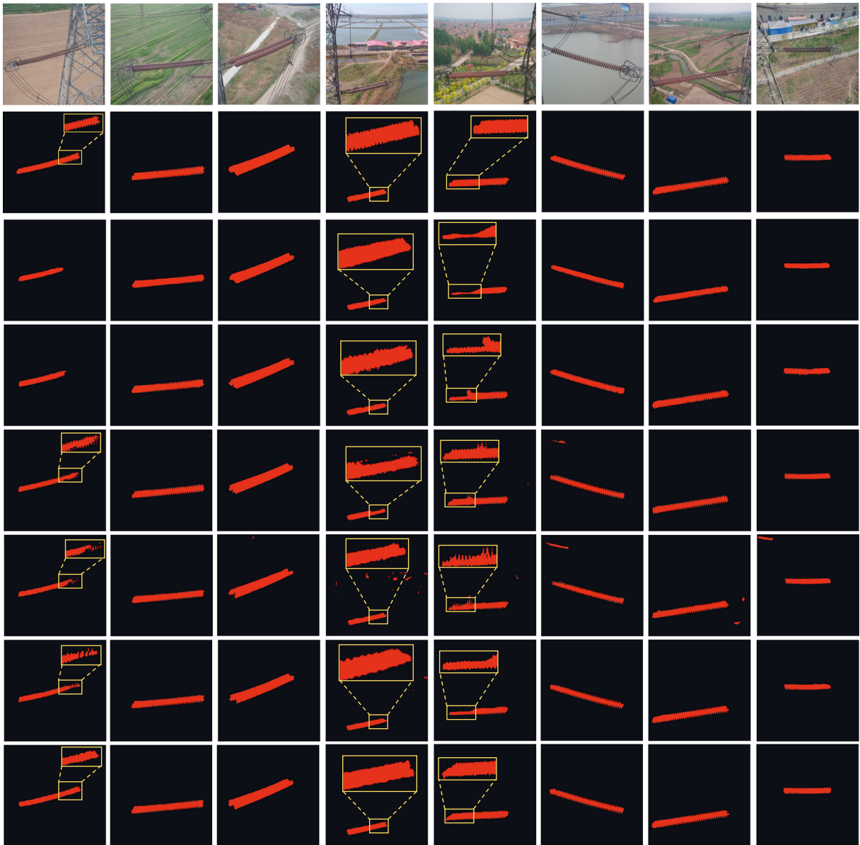
FIGURE 9: In the insulator test dataset, the ROC curves are generated by ED-Net and mainstream segmentation models.
