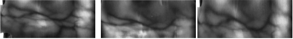
Fig. 2: ROI of sample images of the PLUSVein-FR after applying CPN. Left: palmar view ( 0^\circ ), middle: vein image captured at 45^\circ , right: 45^\circ artificially rotated version of the palmar image.
