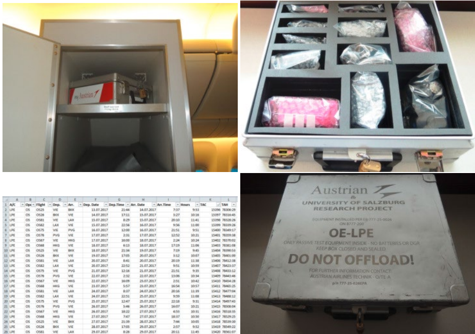
Fig. 1: FP capturing devices situated on the plane: top left - location on the place, bottom left - flight protocol excerpt, top right - capturing devices stored in the aluminium box, bottom right - aluminium box top side.
