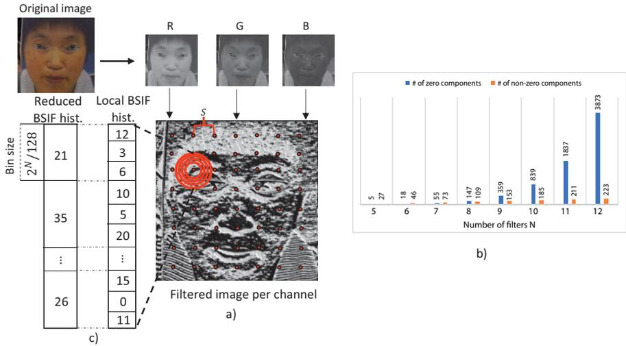
Fig. 2: BSIF feature extraction. a) BSIF histograms are densely computed at fixed points on a regular grid with a stride of  $S$  pixels, b) average number of zero and non-zero components of dense-BSIF histograms for different numbers of filters  $N$ , and c) a reduction example where a local BSIF histogram of size  $2^N = 512$  is represented as a 128-component vector.
