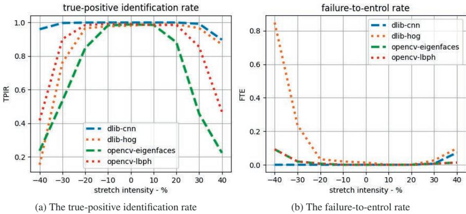
Fig. 2: TPIR and failure to enroll (FTE) from 40% vertical contraction to 40% horizontal contraction
