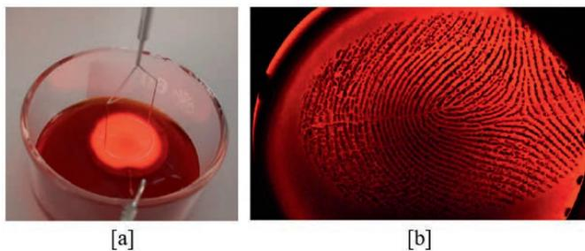
Fig. 1: [a] Experimental setup with recommended chemicals published by *Xu et al.*; Reproduced by our research group [b] high-contrast and high-resolution images of fingerprints based on the method described by *Xu et al.*
