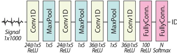
Fig. 2: Architecture of the biometric identification model
