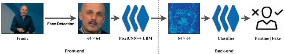
(b) The training and evaluation pipeline of the classifier. The pre-trained anomaly detection model is used as an anomaly feature extractor.
