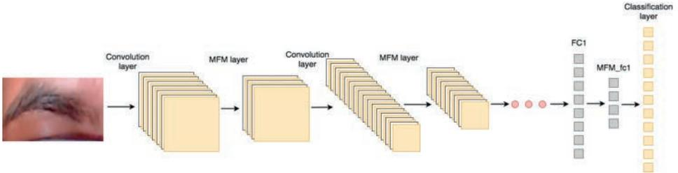
Fig. 3: Architecture of the lightCNN model used in this study.
