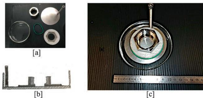
Fig. 2: [a] Overview of the components, [b] construction sketch cross-section and [c] structured analysis cell. The construction as seen in the picture consists of a petri-Dish, they contain two electrodes (stainless steel -plate, -nut), separated by a plastic insulator.
