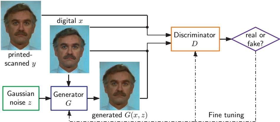
Fig. 3: Concept of the proposed cGAN-based print-scan transformation.
