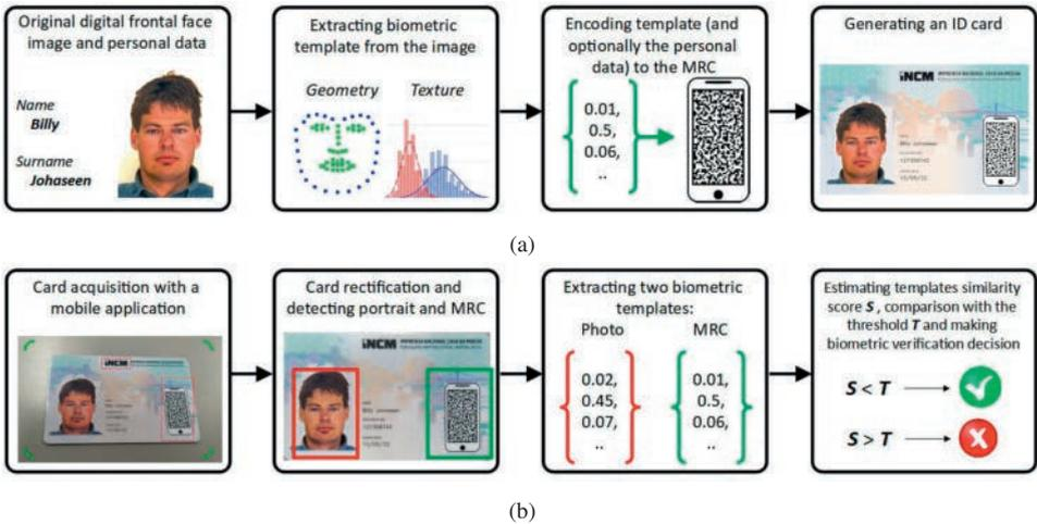
Fig. 1: Pipeline for ID generating(a) and validating(b) in the proposed system.
