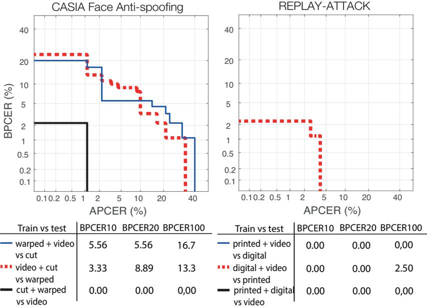
Fig. 3: *Unknown-attacks* DET curves and BPCER(%) values over the leave-one-out protocol for the CASIA and REPLAY-ATTACK databases. The REPLAY-MOBILE database reports a BPCER = 0.0% for any APCER.
