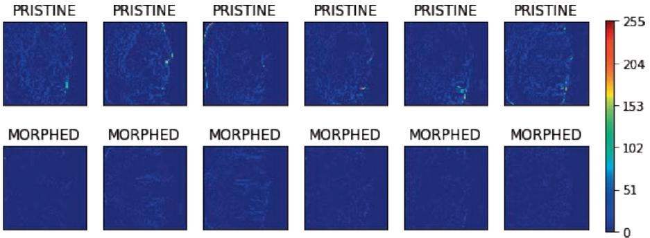
Fig. 4: Example of prediction error *images* of cropped faces in a six-frame sequence of pristine frames (top) and morph-cut frames (bottom) in a video. The images visualize the absolute gray value difference per pixel between the interpolation output and the actual frame.
