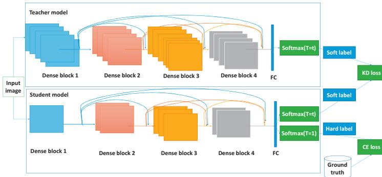
Fig. 1: An overview of the proposed KD approach for periocular verification based on DenseNet architecture.
