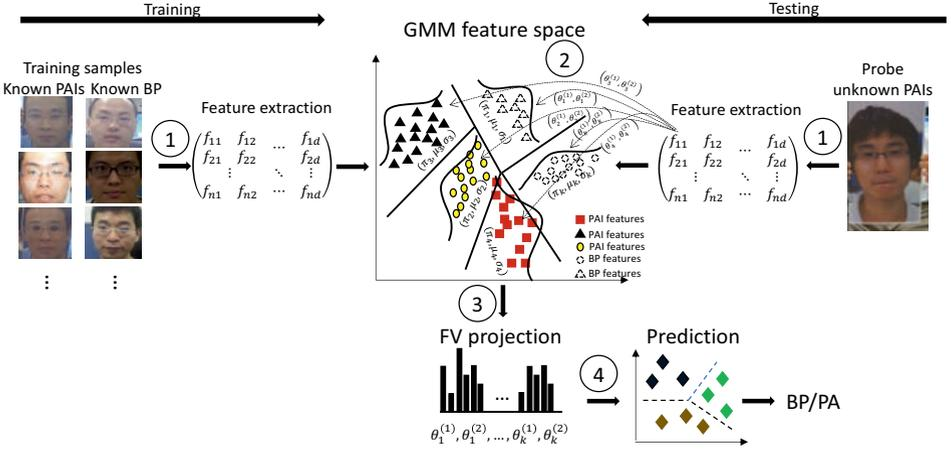
Fig. 1: Face PAD approach overview which comprises three steps: *i*) BSIF descriptors are densely extracted; *ii*) the BSIF data distribution is subsequently learnt by training an unsupervised Gaussian Mixture Model (GMM) from known samples; *iii*) an unknown sample at hand is then encoded by computing the gradient among their BSIF components and parameters obtained by the GMM; and *iv*) the final features are finally classified using a linear SVM.
