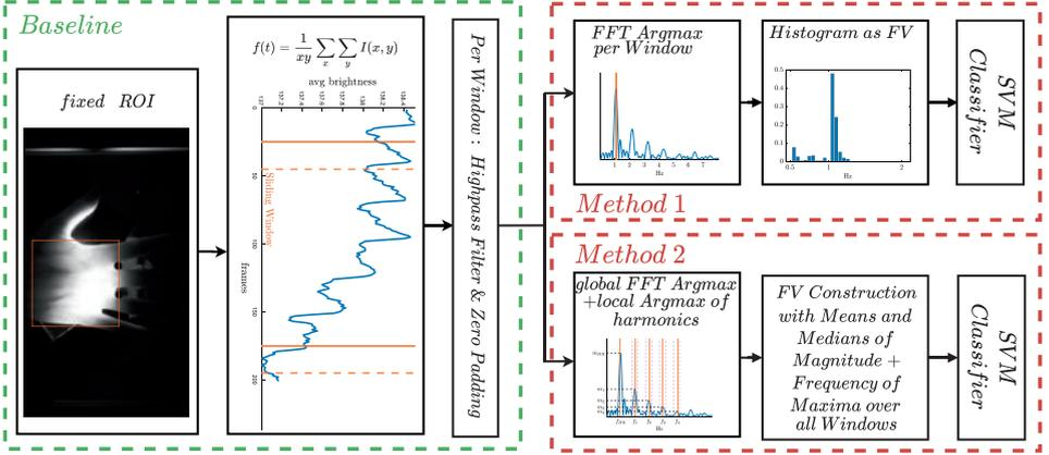
Fig. 3: Block diagram of the proposed methods.
