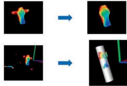
Fig. 4: Estimating ROI using PCL Cylinder Fitting
