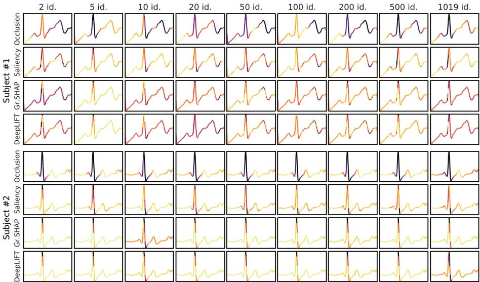
Fig. 6: Average explanations over heartbeat waveforms of subjects #1 (top) and #2 (bottom) on the subsets of the UofTDB database. In each subplot, the yellow to dark purple colours correspond to increasing time sample relevance. Signals were filtered for easy visualisation.
