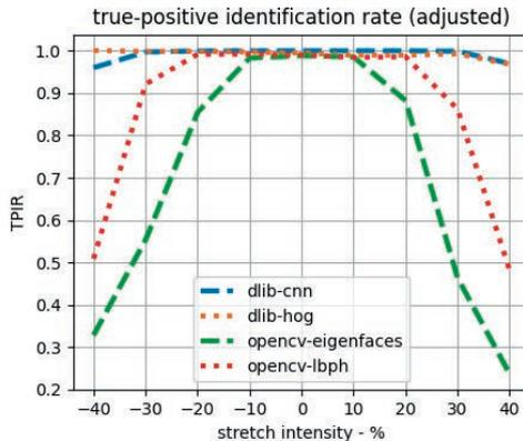
Fig. 3: The TPIR adjusted for FTE
