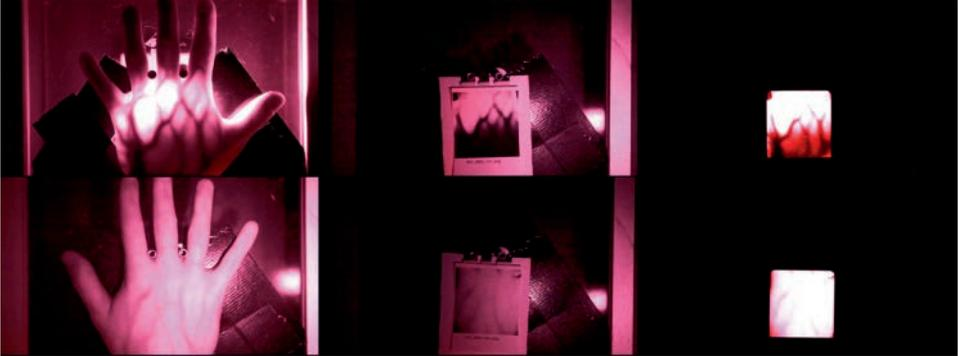
Fig. 2: Example frames from NIR videos; top row: transillumination, bottom row: reflected light; left: bona fide video frame, middle column: paper attack and right: smartphone attack, respectively
