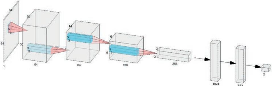
Fig. 2: The diagram of the classifier architecture. Each convolution is followed by a  $2 \times 2$  maxpooling layer and ReLU activation. The network has a total of 933,442 parameters.
