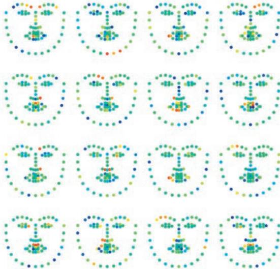
Fig. 7: Facial landmark significance visualization for selected filters in conv1. The significance is measured as the norm of the  $3 \times 3$  matrix corresponding to  $x$ ,  $y$ , and  $z$  coordinates of the landmark in frames  $t - 1$ ,  $t$ , and  $t + 1$ .
