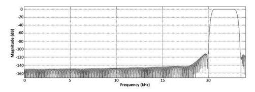
Figure 4: The newly designed bandpass FIR filter (Blackman-Harris window, 20.4 kHz - 23.0 kHz)
