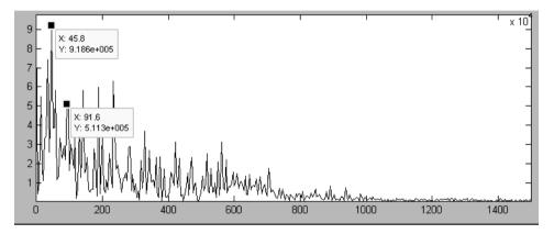
Figure 8: Automatically detecting covert audio signals by frequency shift analysis
