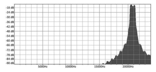
Figure 1: Frequency range (before filtering) of the alternative signal with the ACS modem (FFT, size 1024, Hanning window)
