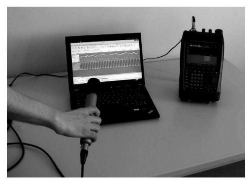
Figure 6: Locating the source of a covert audio signal with a mobile device (PR100)
