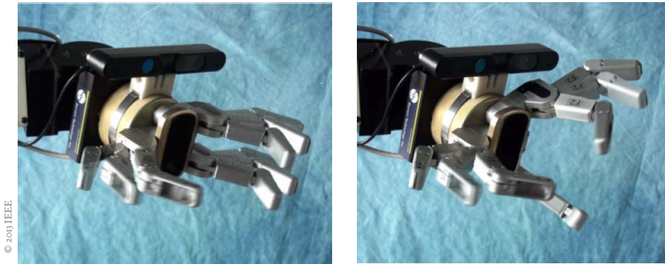
Figure 3.1: The motion of two different compliance modes of the Barrett Hand 262. To find suitable grasps we search for structure that is shaped complementarily.
