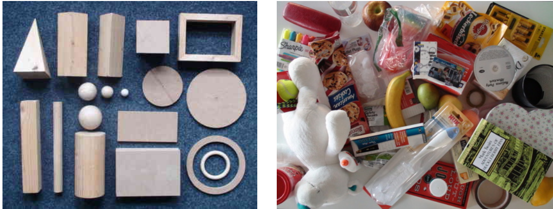
Figure 2.2: We use two complementary object sets for our human-in-the-loop grasping experiments. Left: The first set contains simple geometric shapes such as spheres, cylinders, and prisms. Right: The second set consists of household items such as books, plastic fruits, and stationery. It contains many objects from the 2015 Amazon Picking Challenge (Correll et al., 2016).
