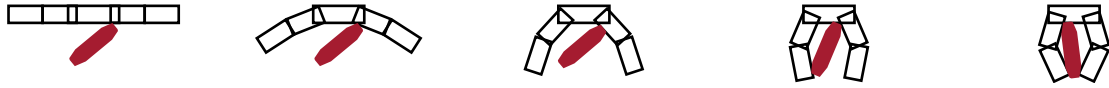
Figure 2.7: To collect evidence for the SFA hypothesis, we simulate vast amounts of grasps with a two-fingered hand in 2D using the daVinci simulator (Berard et al., 2007).
