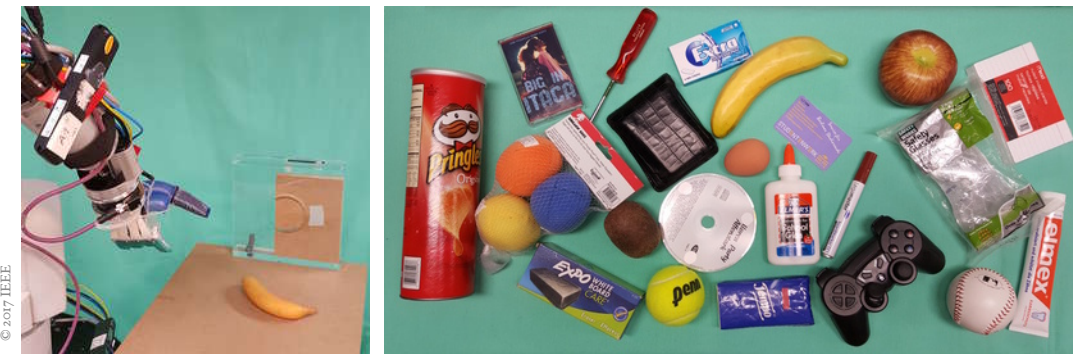
Figure 7.3: Real-world setup for the grasping experiment. Left: Barrett WAM with RGB-D sensor and RBO Hand 2 in front of a table and a vertical structure (transparent). The setup is chosen such that it offers opportunities to do all three types of EC-based grasp strategies. Right: We use 22 different objects in the real-world experiment.
