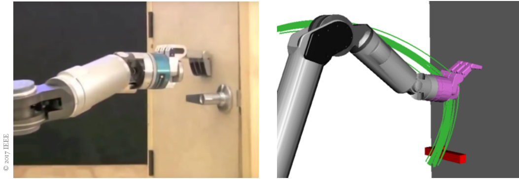
Figure 4.1: Contact can efficiently reduce the uncertainty about the robot’s state. Left: An example from a manipulation challenge, where the robot first touches the door to localize the handle before attempting a grasp (Righetti et al., 2014). Right: A similar strategy, generated by our planner CERRT. Shown in green are several executions of the motion under uncertainty, which all first contact the door and then slide down to the handle.
