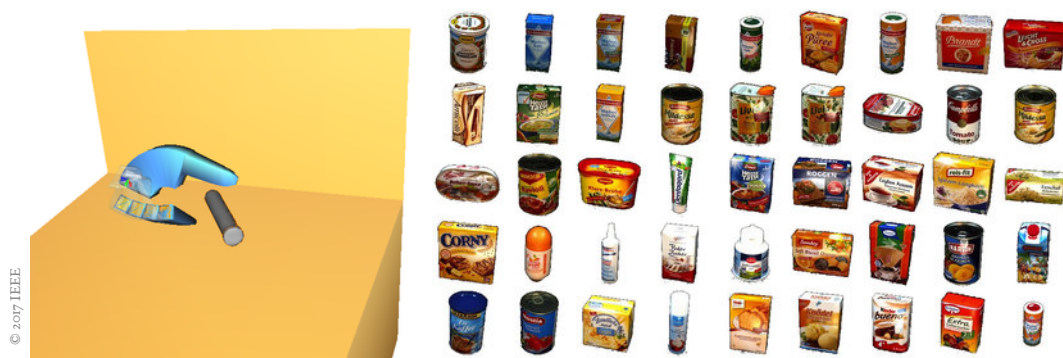
Figure 7.2: Simulation setup for the grasping experiment. Left: Simulated RBO Hand 2 in the SOFA simulation framework. Right: 45 objects from the KIT models database (Kasper et al., 2012). The data set contains a total of 134 objects. The majority of the objects are supermarket products. Since those objects are usually optimized for efficient storage, their geometries do not vary much. Most shapes are cuboids or cylinders.
