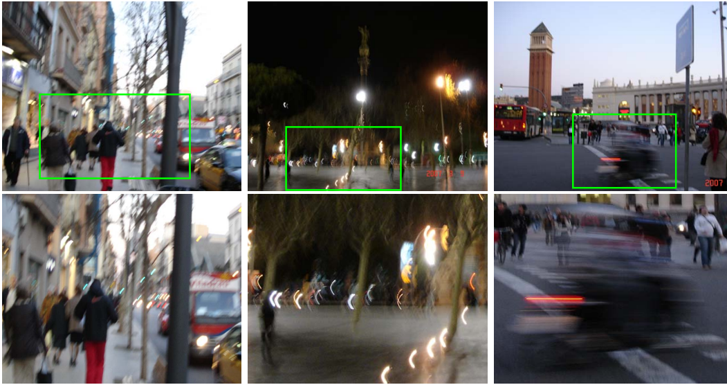
Figure 6.1: a|b|c columns. (a) Entirely, uniform and relatively stationary blurred image. (b) uniform and nonstationary blurred image. (c) nonuniform, partially blurred image.
