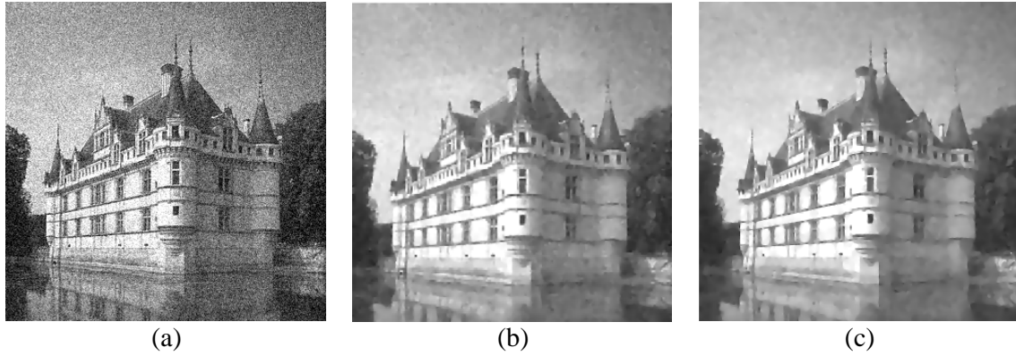
Figure 5.23: Edge-driven denoising. (a) Noisy image with PSNR =25.38dB, sigma = 25. (b) Restored image after 120 iterations. (c) Restored image after 150 iterations
