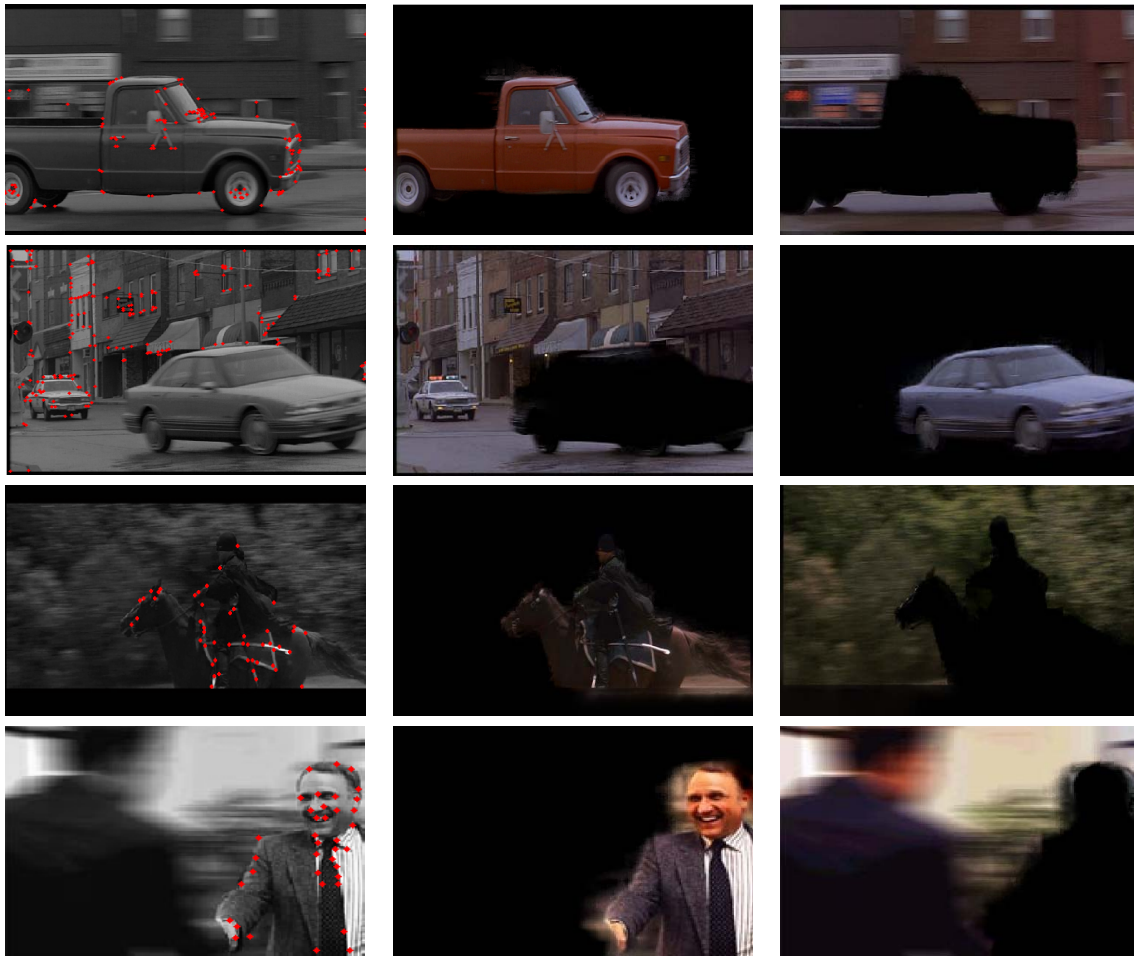
Figure 6.18: a|b|c . Partition and identification of partially-blurred images. (a) Detected feature corners (Föstner operator [79]) as unsupervised prior labeling. These labeling corners can be high-level seeds indicating regions of the image belongs to one regions or object. (b) Segmented unblurred regions or objects. (c) Segmented and identified blurry regions or objects.
