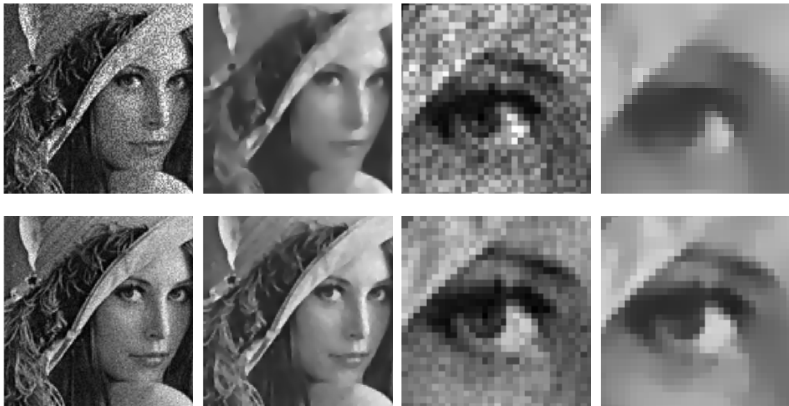
Figure 5.19: \frac{a|b|c|d}{e|f|g|h} . Image denoising using the suggested method. (a)(b) Speckle noise image and denoising. (c)(d) Zoom in from (a)(b) respectively, 100 iterations. (e)(f) Poisson noise image and denoising. (g)(h) Zoom in from (e)(f) respectively, 100 iterations.
