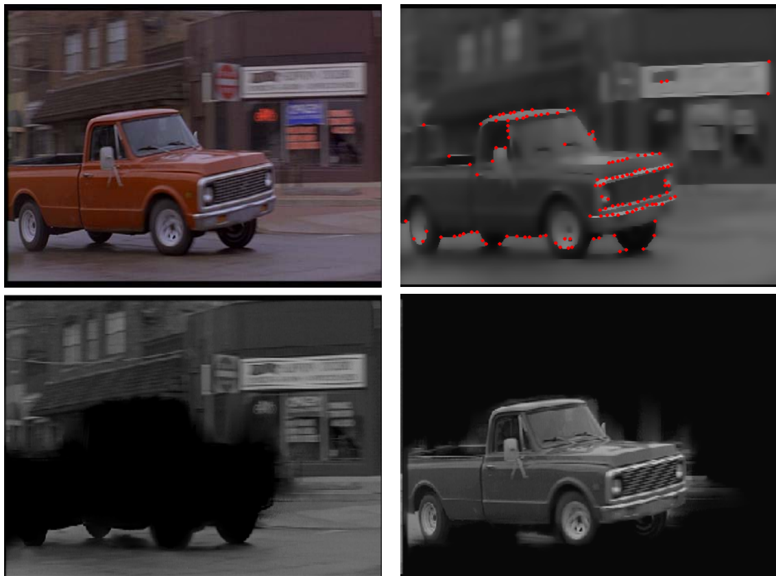
Figure 6.17: \frac{a|b}{c|d} The performance of segmentation for partially-blurred image in pure gray value. (a) Original video data. unblurred foreground car with blurred background. (b) Feature detection after Perona-Malik nonlinear image filtering, K = 10 . (c) Segmented and identified blurred background in gray value. (d) Segmented and identified unblurred car.
