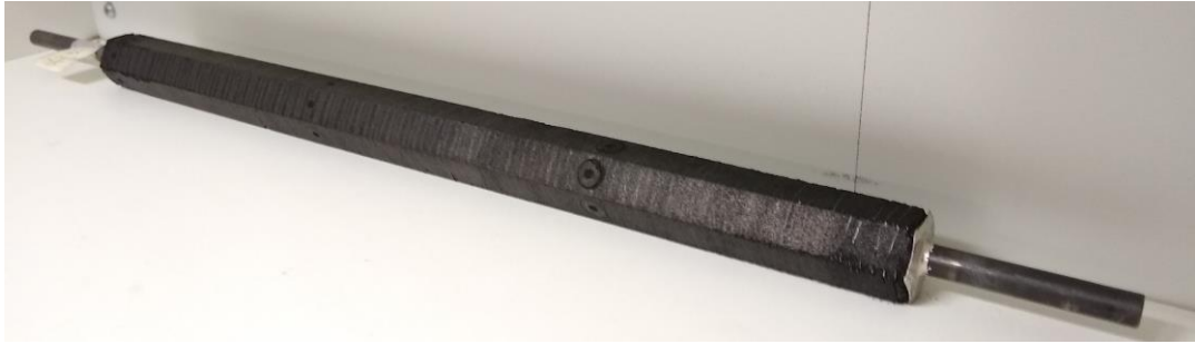
Figure 2 – Generator tube module (19 tubes per generator)
