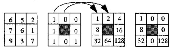
**Figure 6**: The schematic diagram of LBP algorithm when turning image intensity into binary descriptors in 3\*3 pixel neighborhood [18]
