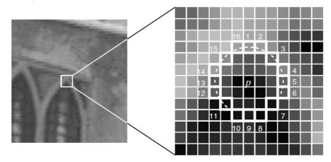
**Figure 3**: The Schematic diagram of sampling area when FAST feature detection algorithm extracts features[21]
