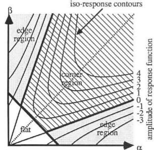
Figure 1: The schematic diagram of the Harris corner detection algorithm to judge the kind of zone[16]
