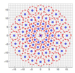
**Figure 8**: The schematic diagram of the concentric sampling pattern used in BRISK algorithm[34]
