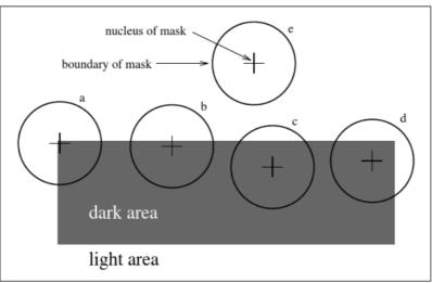
Figure 2: The schematic diagram of the circular window used in SUSAN[19]
