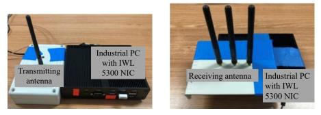
Figure 7: The transmitter (left) and receiver (right) of CSI.
