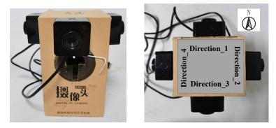
Figure 8: The collect equipment of multidirectional image (Left: front view, Right: top view).
