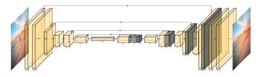
**Figure 3:** Reference architecture for the autoencoder. The input (compromised) image is processed through the convolutional layers and its sanitized version is produced as output.
