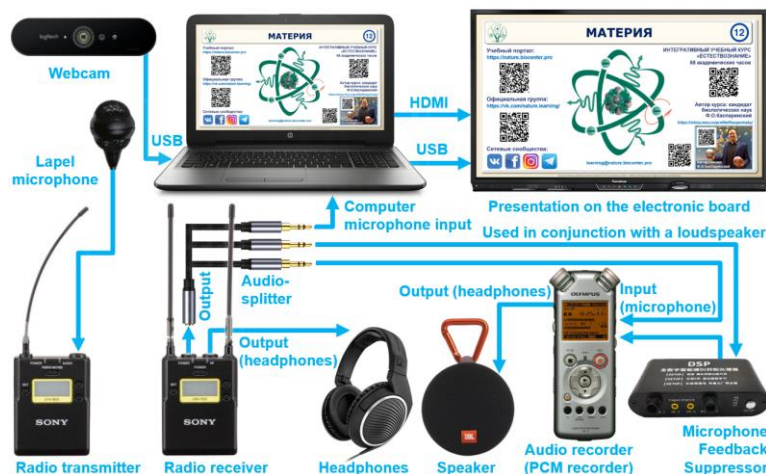
Fig. 9. Connection diagram of audio equipment for computer recording of video lectures in the classroom.
