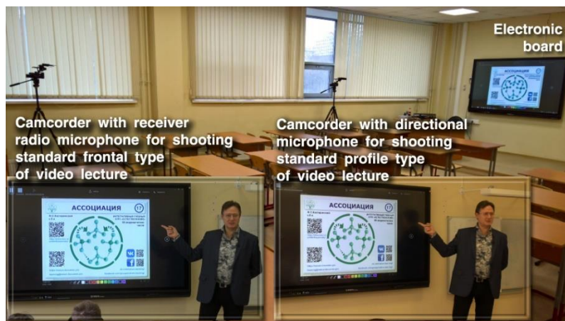
Fig. 7. Placement of video cameras for profile and frontal filming of a lecture in an auditorium with an electronic board.
