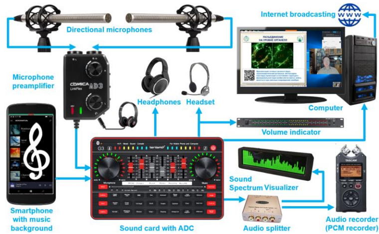
Fig. 15. Audio equipment connection diagram for online teaching.
