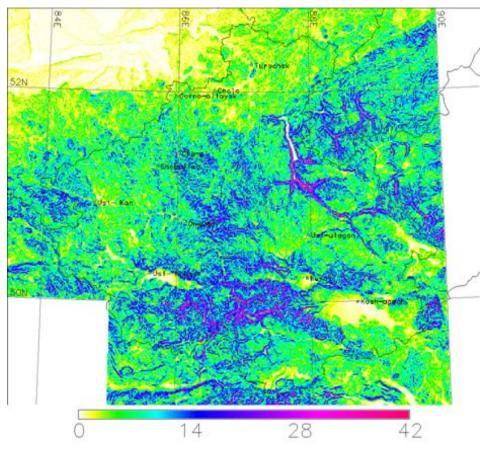
Figure 2. The slopes of the underlying surface for the territory of the Altai Republic obtained according to the digital terrain model SRTM.
