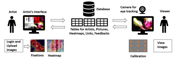
Figure 1. System Architecture: the image depicts the interactions among the three modules: 1) Artist's Interface, 2) Viewer's Interface, and 3) Database
