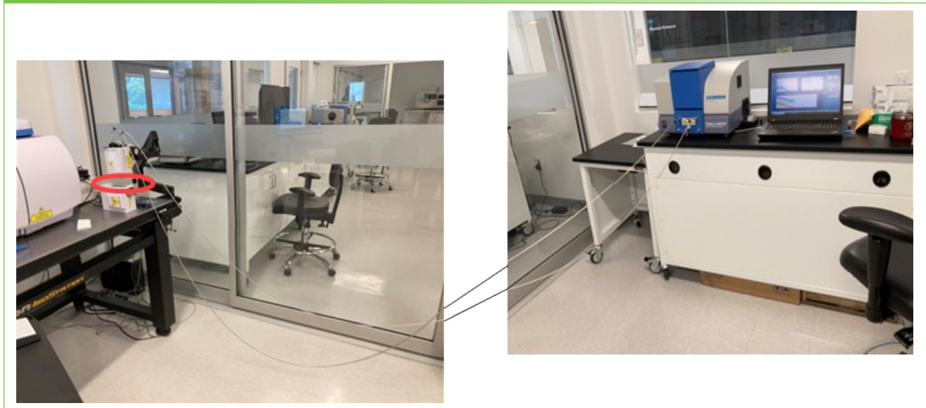
FIGURE 2: The scheme under which the measurements of the epoxy cure were made. The instrument and computer are on one side of the room and the Raman probe is mounted on the other with the fiber optic cables crossing the room. The sample position at the focal point of the Raman probe is noted by the red ellipse on the left.
