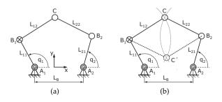
Fig. 13. Kinematic scheme and geometries of the <u>RRRR</u>-mechanism (a) and solutions of the DKP (b).
