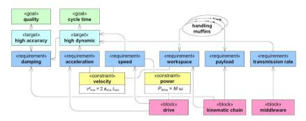
Fig. 4. Elements of an extended requirements diagramm based on SysML.
