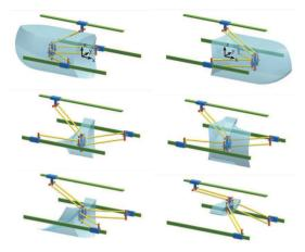
Fig. 11. Main-workspaces in working configuration (top); Selected changeover configurations (middle, buttom) of the TRIGLIDE robot.
