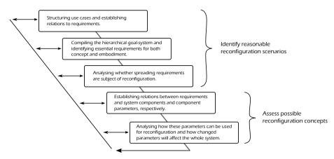
Fig. 5. Working steps for the identification of reconfiguration-relevant parameters.
