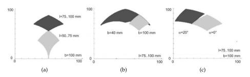
Fig. 8. Influence of the reconfiguration parameter on the position and dimension of the workspace: a) varied strut length  $l_1$ ,  $l_2$ ; b) varied frame diameter b and c) varied angle  $\alpha$  at the frame connection level.
