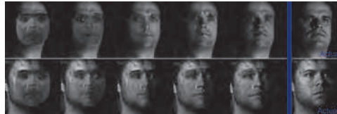
Fig. 8. Evolution of the synthetic face produced by the model during the fitting process, from initialization to convergence.
