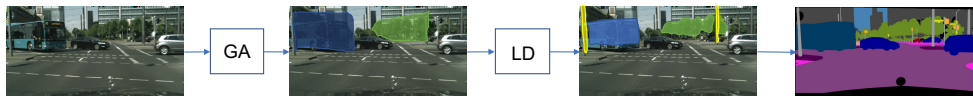
Figure 1: Our proposed GALD framework for semantic segmentation task. The imbalanced spread of information from small and large patterns in GA module is appropriately handled through LD module.
