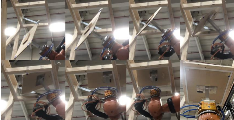
Figure 10 A KUKA KR120 Robot Following Demonstrated Motion Primitives
