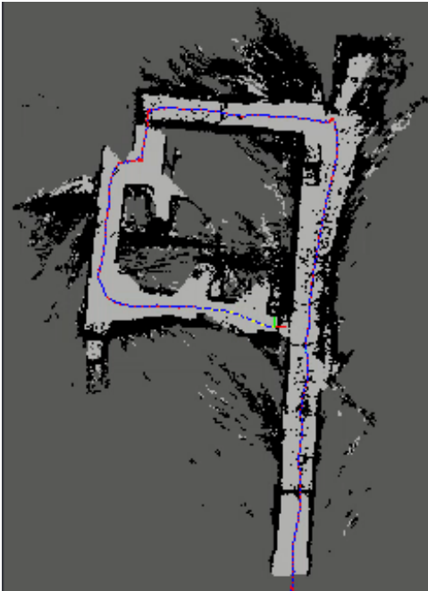
Fig. 15. The wheelchair localizes itself in the mapped environment using the stereo camera data also taking its orientation into account.
