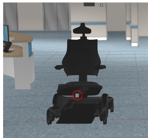
Fig. 9. A detailed model of the wheelchair. The red circle highlights the RGBD sensor mounted on the wheelchair.
