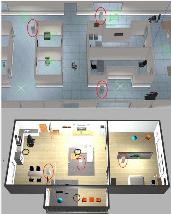
Fig. 10. Both images denote the presence of dynamic obstacles in both hospital and home-like environments. The red circle highlights the dynamic obstacles.
