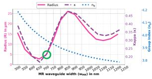
Fig. 3: MR design exploration with the selected MR design (R=5  $\mu$ m) highlighted by the green circle.
