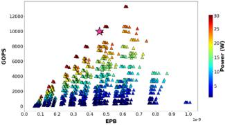
Fig. 6: Architectural exploration analysis for *RecLight*, with the aim to find the optimal [v, N, M, NwG] configuration with the best energy-efficiency and throughput. The best configuration, which is [15, 15, 40, 10], has the lowest EPB/GOPS value and is indicated using a pink star
