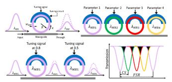
Fig. 1: An MR with tuning circuit (top left) used for tuning wavelengths to reflect parameter values. Such MRs can be placed together to form an MR bank (top right). MRs of the same wavelength can be used to perform multiplication operations (bottom left). The transmission spectrum of an MR bank is shown on bottom right, depicting free-spectral range (*FSR*), channel spacing (*CS*), and inter-channel crosstalk (regions shaded black).
