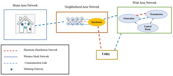
Fig. 2. Main Sub-Networks in the Smart Grid Architecture.
