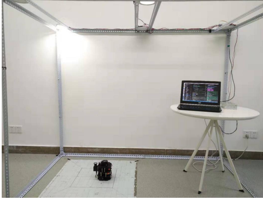
Figure 7. The experimental platform of VLP system based on positioning algorithm.
