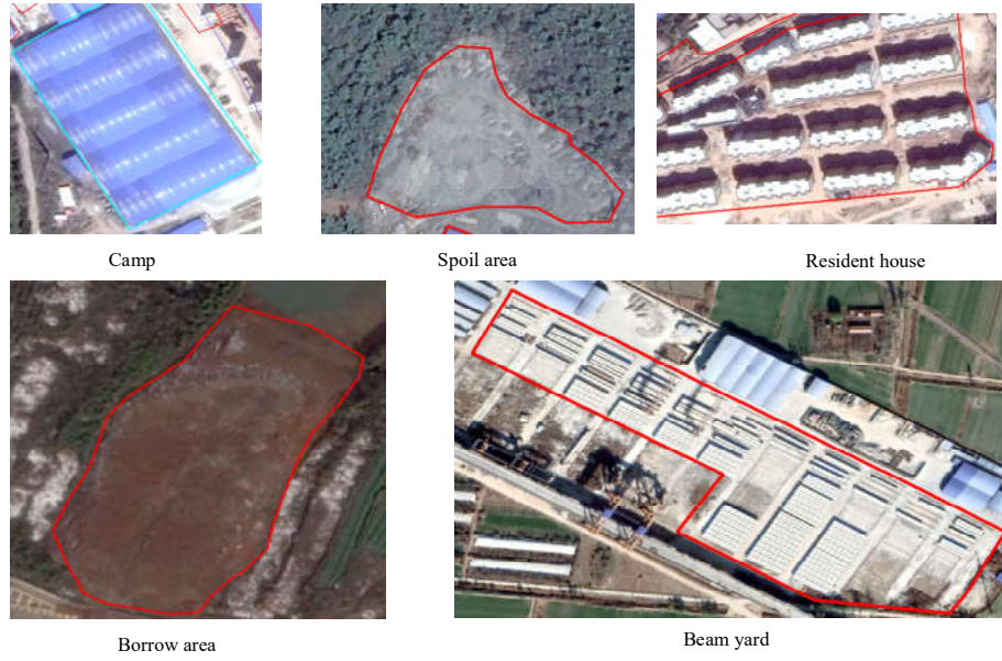
Figure 1. Visual appearance of the target temporary works and ESAs in VHR images
