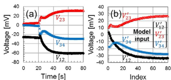
**Figure 3** (a) Raw differential voltage data and (b) processed data for training of machine learning model. The multi-array sensor was displaced from a 0.1 M KCl reference solution to the sample solution at 20 s, in this example a soft drink “beverage B”.
