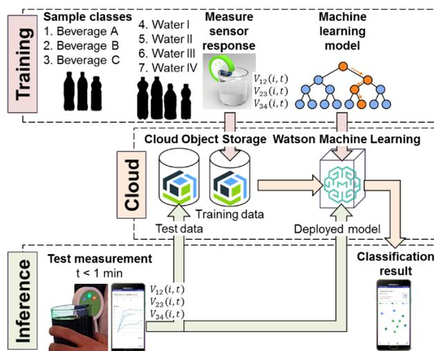
**Figure 2** Workflow for the portable electronic tongue device depicting stages for training and inference, along with cloud computing services for storing training and test data as well as execution of trained machine learning models during inference.
