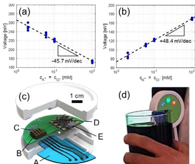
**Figure 1** (a) Anionic sensitivity of electrodeposited PPy films with change in KCl concentration, (b) cationic sensitivity of electrodeposited PPy/FOCN films with change in KCl concentration, (c) assembly of sensor array on PCB [A] with spring-loaded connector [B] and read-out electronics comprising an ADC [C] and microcontroller [D] with micro-USB port [E] for connection to smartphone, and (d) photograph of packaged electronic tongue device immersed in liquid sample.
