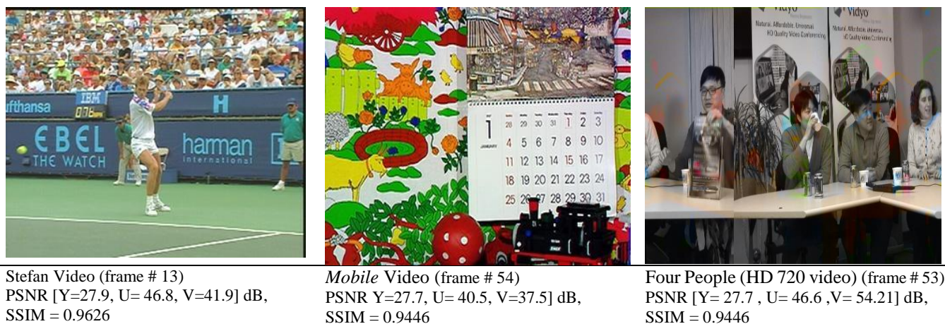
Fig. 5 Videos frames from the test videos (without crypto-transrating) showing PSNR and SSIM values for the luminance, Y, and chrominance, U and V, components
