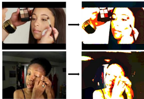
Figure 3 Example of segmented images from action 'Apply Eye Makeup' of UCF101 dataset. First row images are from subject 04 whereas the second-row images are from subject 25. It can be noticed that segmentation removes the visual bias of skin color from both subjects.
