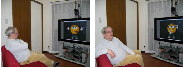
Figure 1: With the iMime system non-verbal interaction is driven by data about a subject's gaze, gestures, and motion qualities as observed using video input from multiple cameras.
