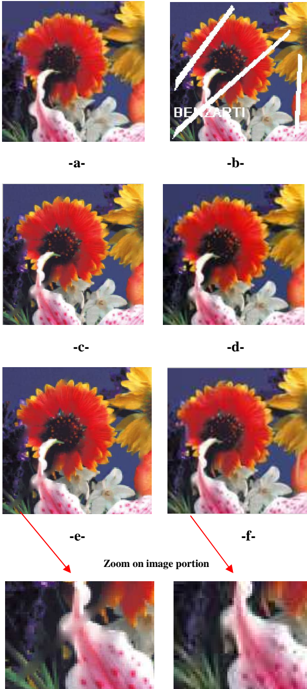
Fig. 6 Test on real photographic image,-a- Original image, -b- Damaged image,-c-TV inpainting method, -d- Fast Inpainting method -e- Harmonic inpainting method,-f- Proposed method
