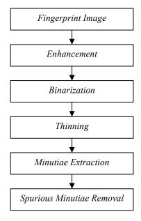
Figure 2. Block Diagram of FVGFE
