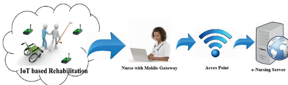
Figure 5. Proposed IoT-based communication architecture for BSN-Care+.
