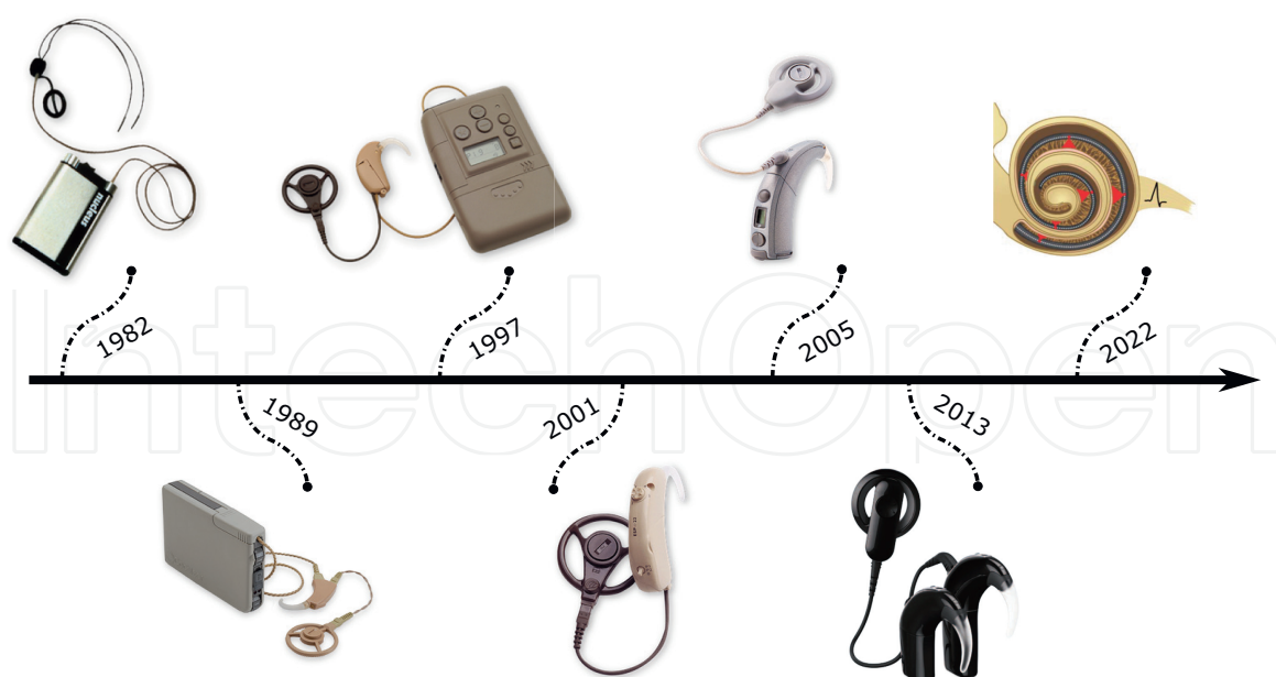
Figure 1. The evolution of CIs from 1982, when the first CI manufacturing company was founded, until the current state-of-the-art research that validated the feasibility of optogenetics-enabled optical CIs.
