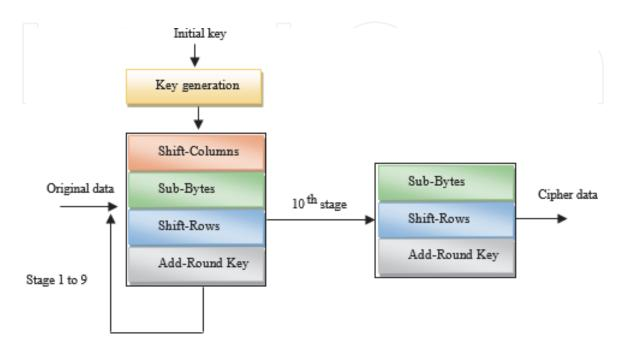
Figure 1. Flow design of AES algorithm.
