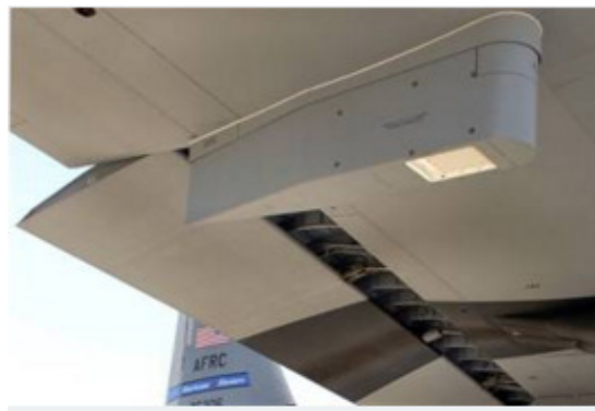
Figure 10, Stepped Frequency Microwave Radiometry
