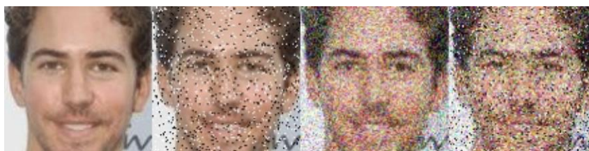
Figure 5. Preprocessed images with noise. From left to right, pure, impulse noise, gaussian noise and mixed noise.
