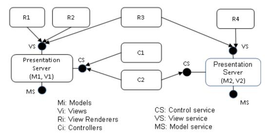
Figure 2. Separation of View-Renderer-Controller in a presentation system.
