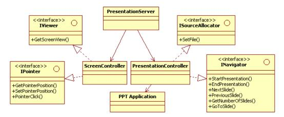
Figure 3. Interface and class definition of the system.
